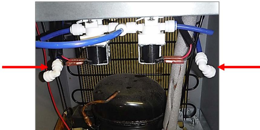
9. Reconnect Tubing into Outlet Elbows once drained.
