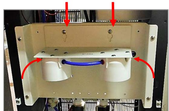
5. Disconnect tank line feed lines from hot and cold inlet solenoids at rear of filter head fittings).
