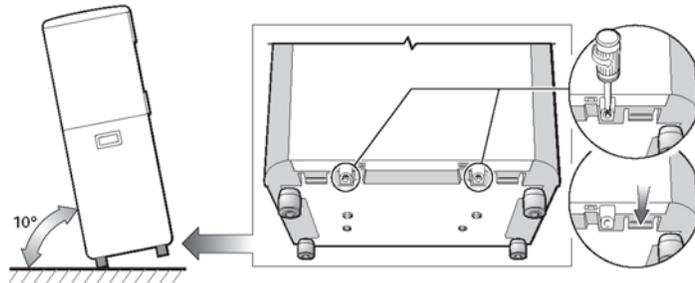
4. Loosen the two screws holding the filter head bracket to remove filter head bracket to access rear of filter heads.
