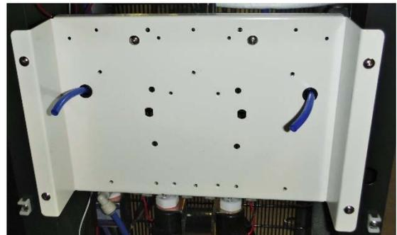
7. Reconnect tubing into inlet elbows once drained, and reinstall the filter head bracket.
