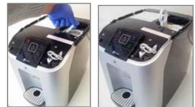
7. Pull the lever straight up to remove the filter assembly. Slight force may be required.
