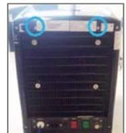
4. Remove the Top Cover by placing your hands on the Top in the picture and push it backwards and then lift it up to remove.
