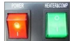
28. Ensure green heater / compression switch is in the O=OFF.
