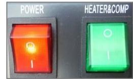
Prior to draining the Hot Tank, turn off Green Heater/Compressor Switch (O=OFF) located on back of the *CUBE Water Treatment System*
